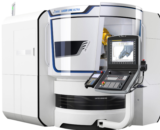
Figure 1: The EWAG LASER LINE ULTRA. A laser-based machining centre equipped with 5 CNC and 3 optical axes enabling it to process practically all materials and geometries without significant thermal input. Source: EWAG
